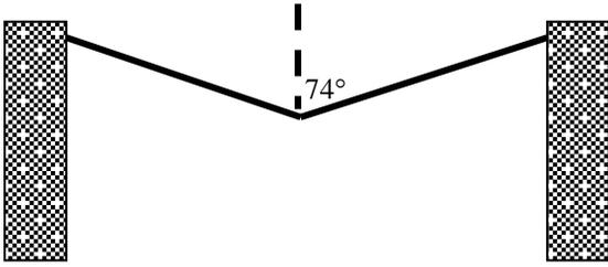
5. The 4.5 N object below is in static equilibrium on the ramp. What is the frictional force that is keeping the object in place? What is the normal force?
