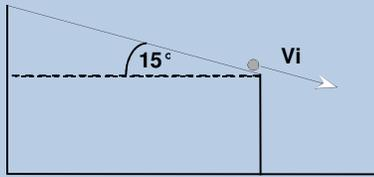
Suppose that the sphere leaves the ramp at  $1.5 \text{ m/s}$ . The bottom of the ramp is  $0.90 \text{ m}$  above the floor. Calculate the range of the sphere.
