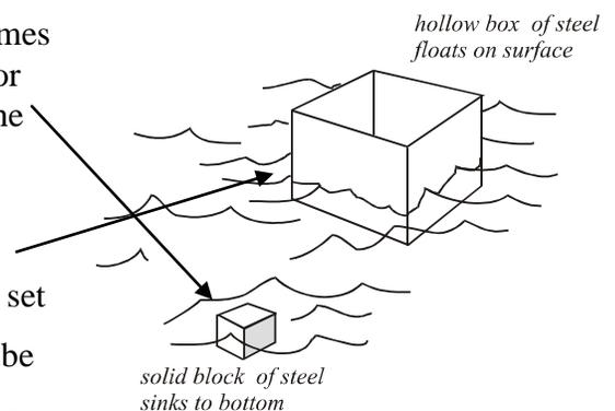
As cargo ships are loaded with freight, they sink deeper into the water. As they sink deeper, they displace more water. This increases the buoyant force. The boat's weight and the buoyant force are at equilibrium. The upward buoyant force is equal to the weight of the ship. As long as the total weight of the ship does not exceed the weight of the water displaced, the ship will float.
