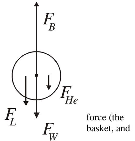
The forces are:  $F_B$  (buoyant force),  $w$  (weight of bag and basket),  $F_{He}$  (weight of helium), and the lift (lifting force)  $F_L$  (weight that is to be lifted).
