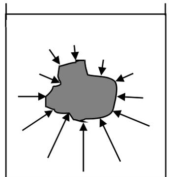
This is because the bottom of the rock is at a greater depth than the top of the rock, so the pressure is greater. Recall that  $P = \rho gh$ , so the greater the depth the greater the pressure. The difference in the forces on the top and bottom are responsible for the buoyant force.
