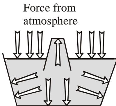
The weight of the atmosphere pushes down on the surface of the water – the old atmospheric pressure. The water in the tub is confined so the pressure exerted on the surface is transmitted throughout the liquid. The pressure exerts a force perpendicular to the surfaces in the tub and in the glass. So the water in the glass is pushed upward.
