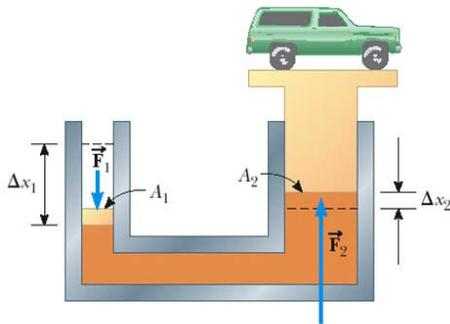
An important application of Pascal's principle is the hydraulic press. The force  $F_1$  is applied to the side with a small area and because the pressure remains the same, that pressure is now applied to the other side with a larger area. The end result is a larger force acting on the car.
