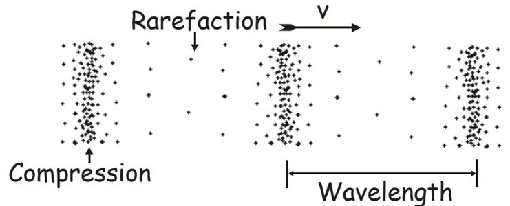
Sound waves are frequently graphed with pressure on the  $y$  axis and time on the  $x$  axis. This makes the wave look like a transverse wave - a sine wave shape on the graph. But in this depiction, changes in pressure are being plotted vs. time and it is not a depiction of the disturbance itself, which is longitudinal. So please, don't be confused between the actual wave and a visual representation of it on a graph.
