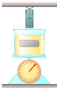
A 2.0 kg beaker containing 3.0 kg of oil (density =  $916 \text{ kg/m}^3$ ) rests on a scale. A 5.0 kg block of iron is suspended from a spring scale and is completely submerged in the oil. Find the readings of both scales.
