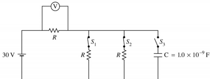
Three identical resistors, each with a resistance of  $2 \Omega$ , and a capacitor of  $1.0 \times 10^{-9} \text{ F}$  are connected to a 30 V battery with negligible internal resistance as shown to the left. Switches  $S_1$  and  $S_2$  are initially closed and switch  $S_3$  is initially open. A voltmeter is connected as shown.
