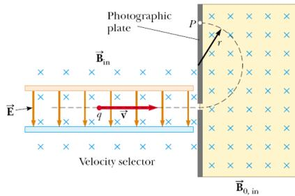
A charged object enters the region to the left and moves at a constant velocity between the two charged plates that are 10.0 mm apart and have an electric potential of 12 V. There is also a magnetic field in this region that has a magnitude of 0.35 T. When the object enters the region after the charged plates a magnetic field causes the particle to follow the path of the dashed line. This path has a radius of 10 cm. (a) What is the strength of the electric field? (b)
